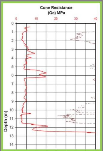
This graph shows a medium dense layer at around 6m, below which is soft soil until around 12.5m which is good founding material. Information used with permission from P.J. Yttrup and Associates who can be contacted on 03 5243 3388 or admin@yttrup.com.
