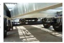
The cross members are a single piece, fully welded to the main vertical web and the coaming rail.
